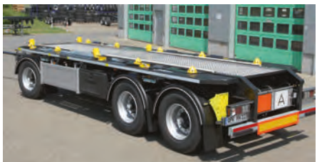
Aluboden am Vario-Carrier
