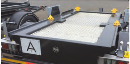
Alu Boden am Mini-Carrier
